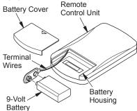
Figure 17 - Installing Battery in Hand-Held Remote Control Unit
